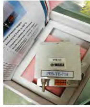
BAROMETER Maker: VAISALA Model: PTB110
