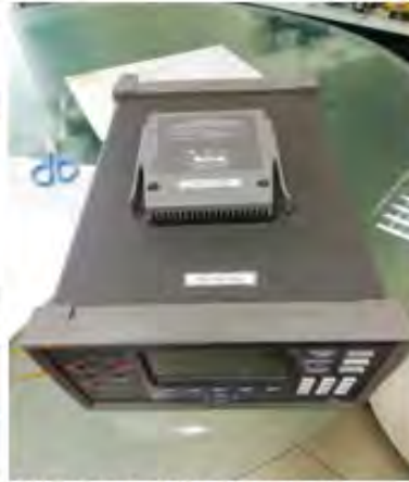
HYDRA SERIES III DATA ACQUISITION W/ INPUT MODULE Maker: FLUKE Model: 2638A
