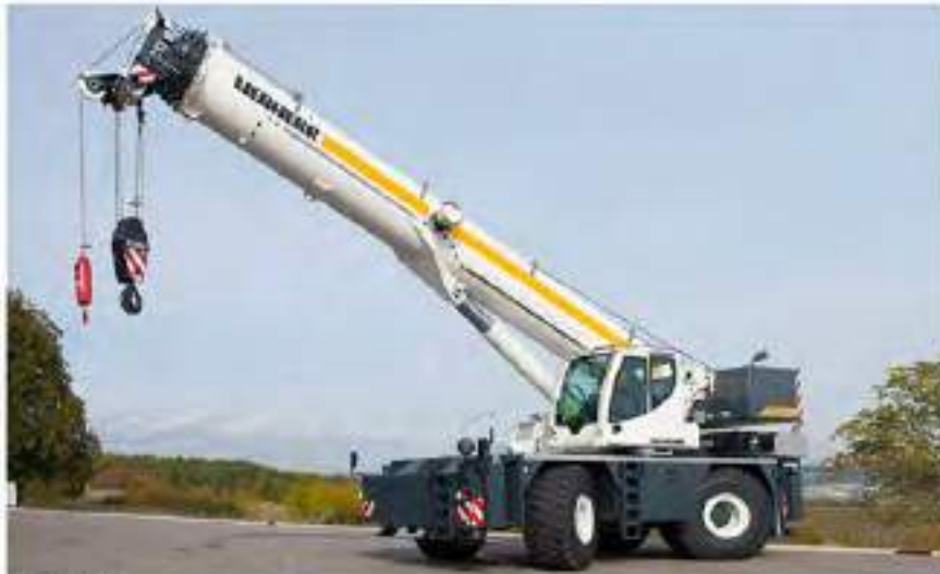
Mobile Crane Rough Terrain 90 tons 'Liebherr' 'S'
