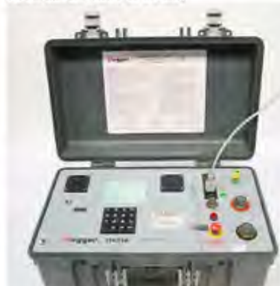
THREE PHASE TRANSFORMER TURN RATIO TESTS
