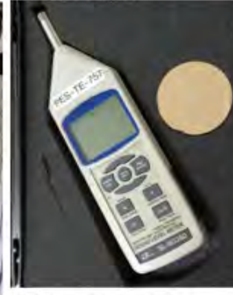
SOUND LEVEL METER WITH CALIBRATOR WIND SHIELD Maker: LUTRON Model: SL-40335D
