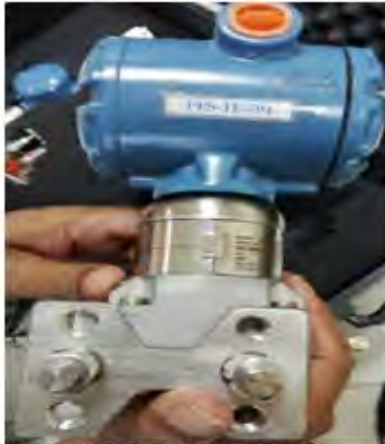
PRESSURE MEASUREMENT TRANSMITTER Maker ROSEMOUNT Model: 3051S1CD12A12A12A1AQ4
