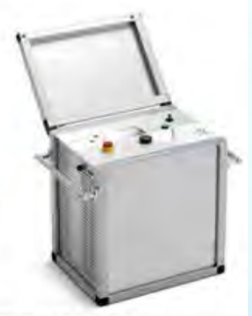
VLF Test Kit ,60kV
