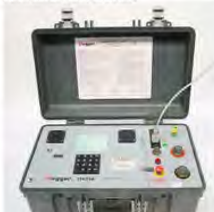
THREE PHASE TRANSFORMER TURN RATIO TESTS
